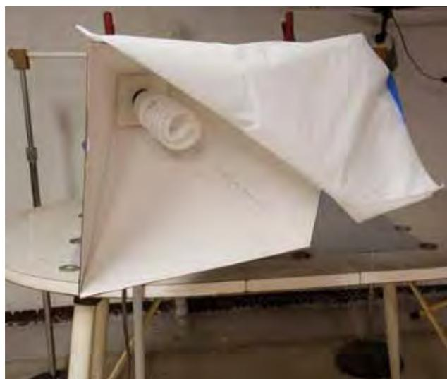
(Above) Diffuser — Made from ½" square strips of wood, covered with a double layer of white plastic tablecloth, the open back side of the diffuser permits the background to curve up behind the object so that the light intensity falls off. The result is a softly graduated background that fades toward black as it recedes.
