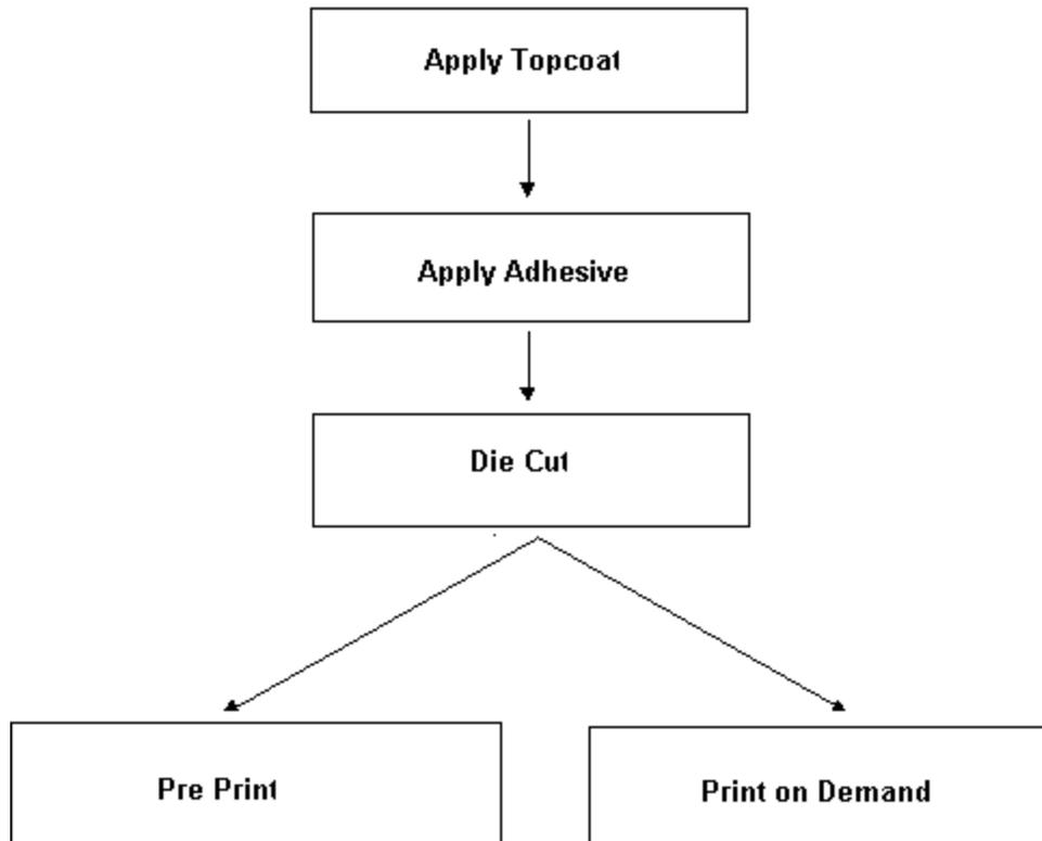
**Figure Two: Flow chart of the typical label manufacturing process.**
