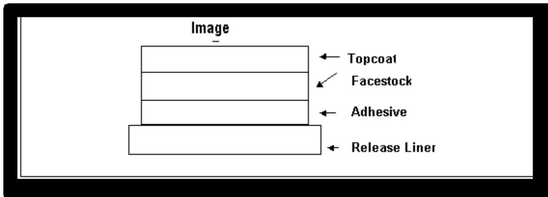
Figure 1: Cross Section of a Pressure Sensitive Label
