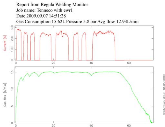
FIGURE 3. UNREGULATED GAS FLOW CONSUMPTION.
