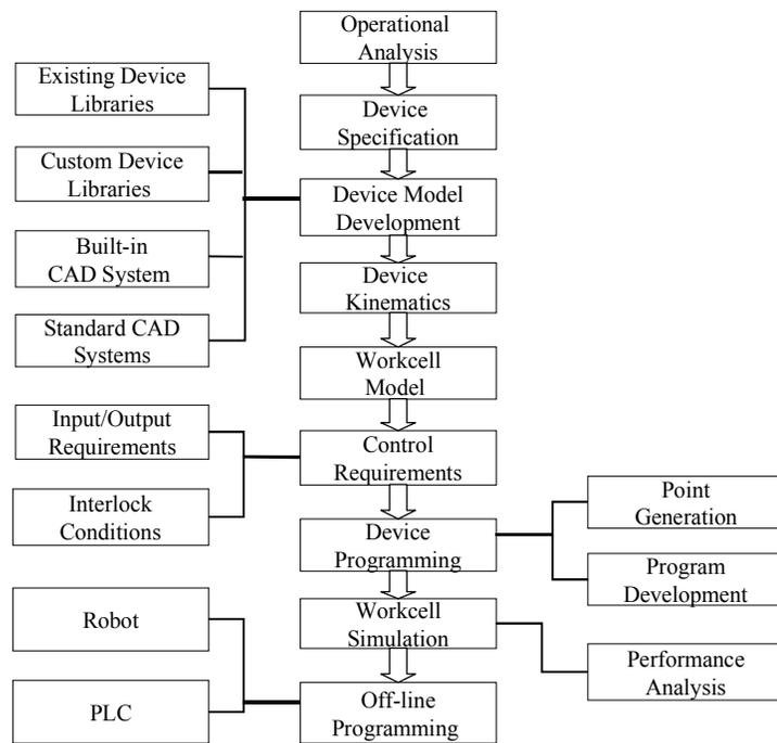
**Figure 1. Flowchart of Workcell Simulation Using Deneb/IGRIP Software**
