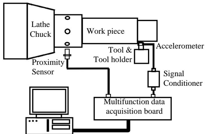
Figure 2. Wiring of the signal system
