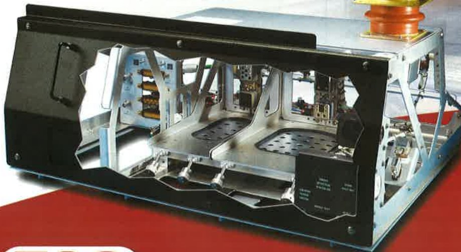
Cutaway view of a Fully Integrated GSM Overhead Storage Compartment Installation Rack for Single Aisle aircraft.
