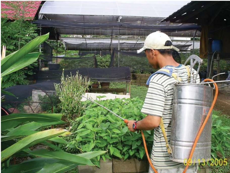
**The Backpack Sprayer is standardized in Asia. It holds 4 gallons or 15 liters and is easy to repair. We can always find replacement parts. It can be refilled efficiently and is economical; one man can cover up to 2 hectares using this clever invention.**
