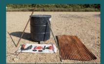
**Tools**: Drill, drill bits, plyers, string, marker **Materials from recycling**: barrel, 2 sheets of roofing metal, 2 m 1" steel box,
