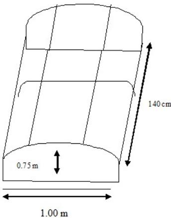
**Figure 3: Plastic tunnel design for MMN**
