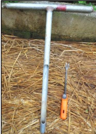
Figure 2 Soil corer for soil sampling (fabricated in a machine shop in Chiang Mai)
