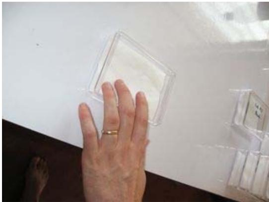
**Figure 4:** With sterile hands or tweezers, fit cut paper towel into petri dish#
