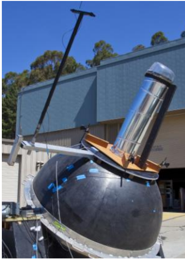
Figure 8-1. Photograph of integrating sphere with TDD installed.
