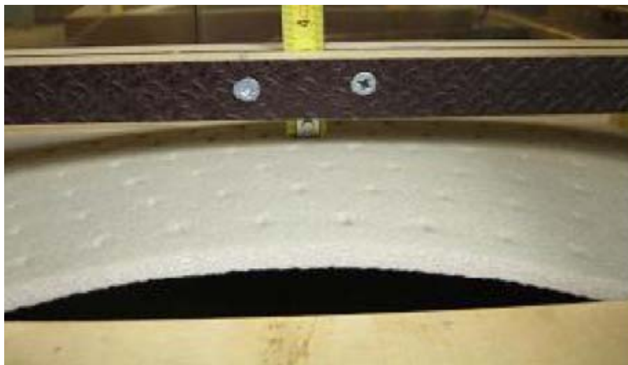
Figure C.3 – example of shockpad bowing (concave)
