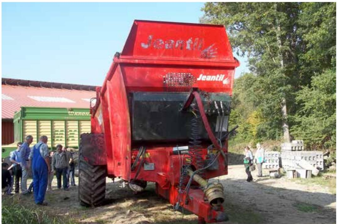
Spreader used for putting digestate onto the fields.
