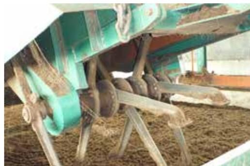
*Aeration tynes on the compost making system for turning compost.*
