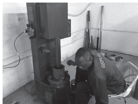
Execution of Modified AASHTO density test in order to determine Maximum dry density (MDD) and Optimum moisture content (OMC)
