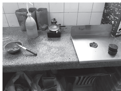
Apparatus utilised to determine the Atterberg limits The Atterberg limits apply to the soil fines (<0.425mm)
