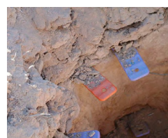
Figure 2. PRS probes in place on the Virgin River floodplain, in the soil profile.
