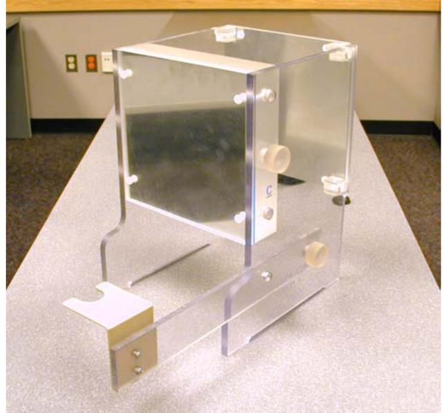
A fully assembled phantom
