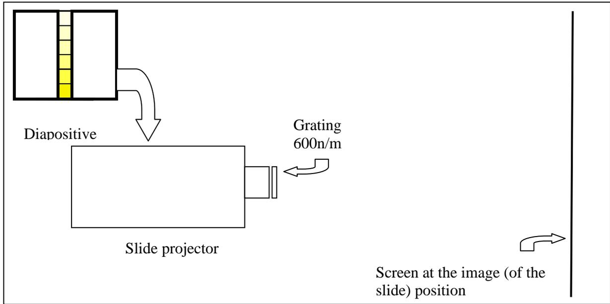
Figure 2. Sketch of the setting used to make the spectra shown in Figure 3
