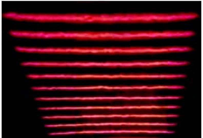
Figure 8: Image of a concrete surface being illuminated by an 11-line generator
