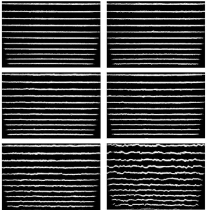
Figure 9: Laser profiles for the 6 different roughened concrete surfaces of Figure 5
