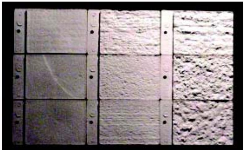
Figure 3: Plastic model concrete surface profiles. The profiles are ordered 1 to 9 in order of increasing roughness, and correspond to acid etching, grinding, light shotblast, light scarification, medium shotblast, medium scarification, heavy abrasive blast, scabbing, and heavy scarification
