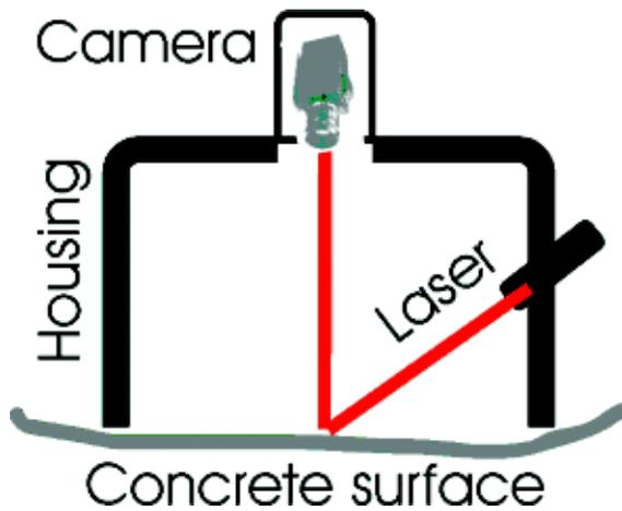
Figure 4: Schematic representation of the laser-profiling equipment
