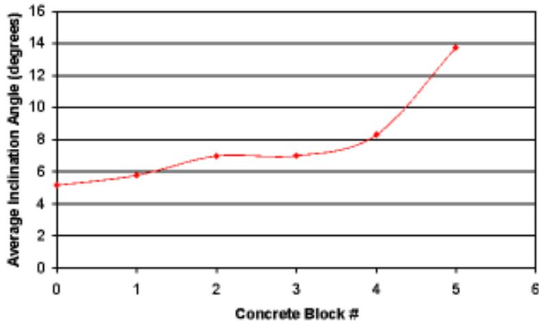
Figure 10: Roughness measurement results for the six concrete surfaces in terms of the average inclination angle of the profiles
