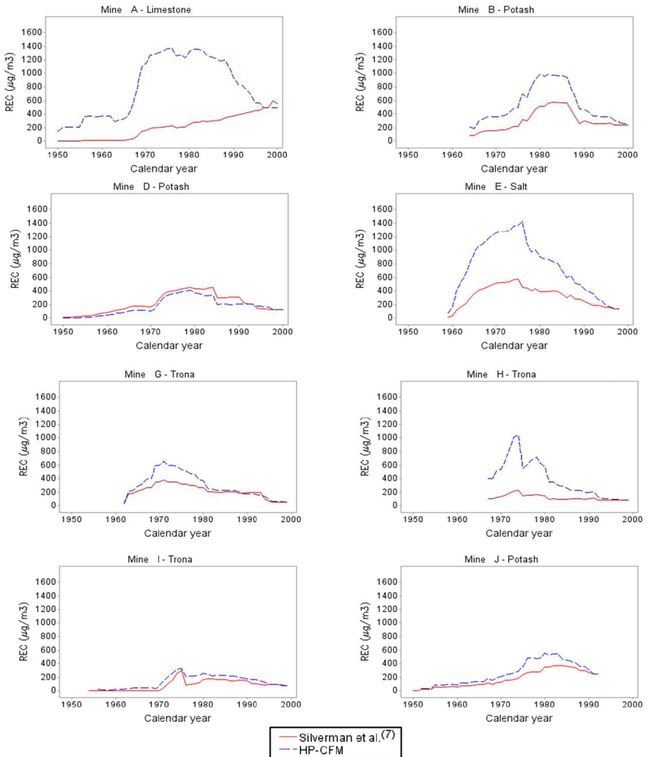
**Fig. 3.** Graphs of mine-specific yearly estimates of REC for mine operators (load operators for mine A) used by Silverman *et al.*<sup>(7)</sup> based on using CO as a surrogate for REC, compared with corresponding REC estimates (labeled “HP-CFM”) developed herein using diesel engine horsepower by year for each mine, the relationship between model year and PM emissions per HP shown in Fig. 2, and mine-specific ventilation rates by year, and which do not rely upon CO data.
