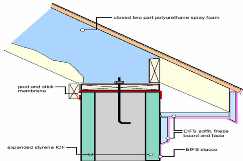
Figure 5 Schematic design of a wall –roof connection
