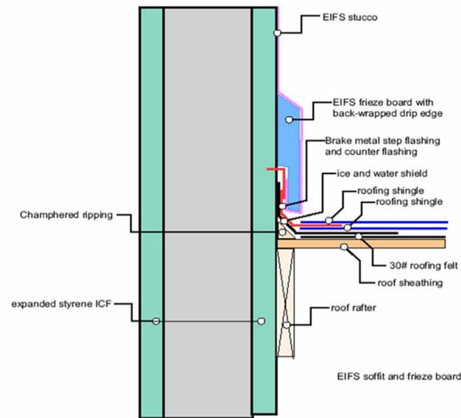
Figure 6 Schematic design of a wall – deck connection
