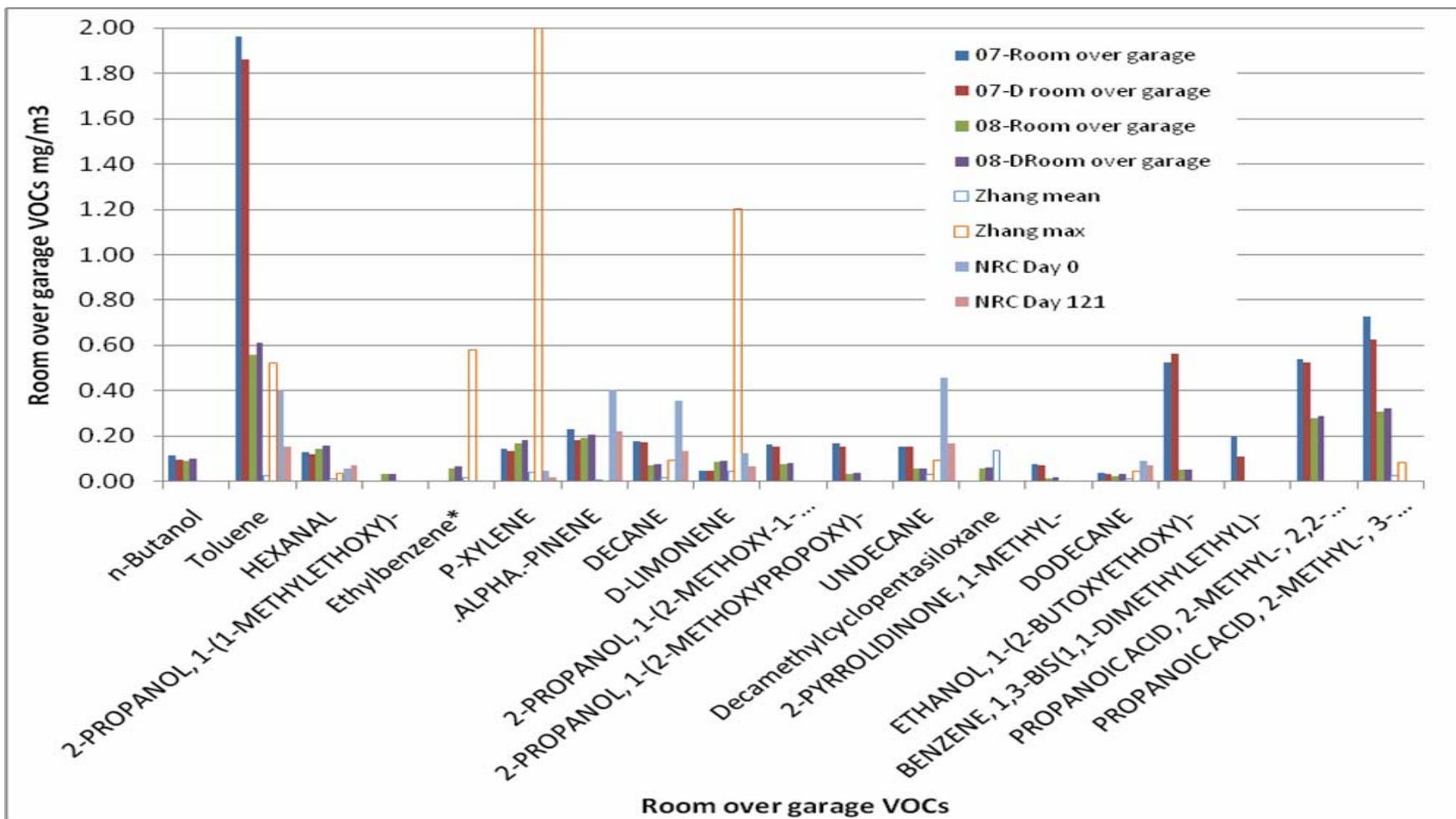
Figure 14. VOC results from measurements performed in Bonus room (over garage) insulated with Spray Polyurethane Foam.
