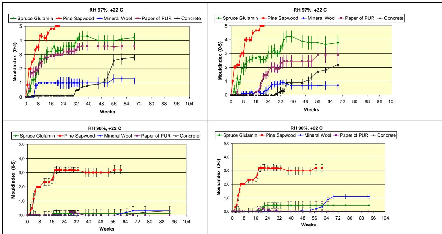
Figure 1. Response of some building material to mould growth at RH 97 – 98 % / 20 °C (above) and RH 90 % / 20 °C (below). For some materials, the response has been higher on the upper surface subjected to mould suspension (left) than that on under side surface (right).
