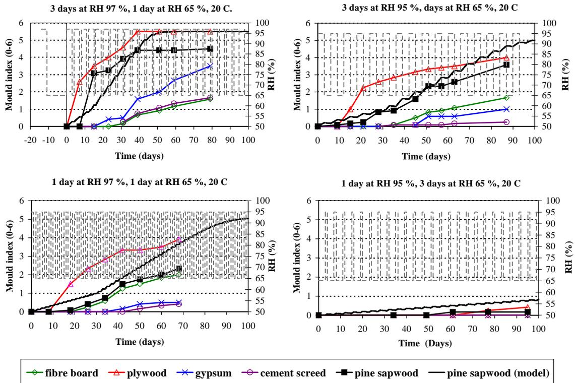
Figure 4. The susceptibility of the different building materials to mould contamination at fluctuated humidity conditions at +20 °C. 3 days at RH 95 % / 1 day at RH 65 %, 3 days at RH 95 % / 3 days at RH 65 %, 1 day at RH 95 % and 1 day at RH 65 %, 1 day at RH 95 % and 3 days at RH 65 %. The fluctuating of humidity is shown in the figure as a RH (%) line (Viitanen and Ojanen 2007).
