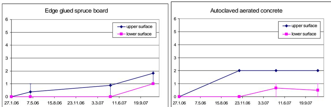
Figure 3. The mould index curves of edge glued spruce board (on the left) and autoclaved aerated concrete (on the right) in field conditions.
