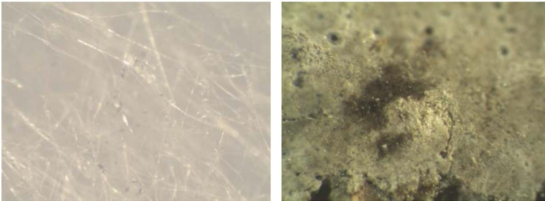
Figure 2. Mould hyphae bonded with glass wool fibres (on the left). Dark *Cladosporium*-mould hyphae in concrete (on the right).
