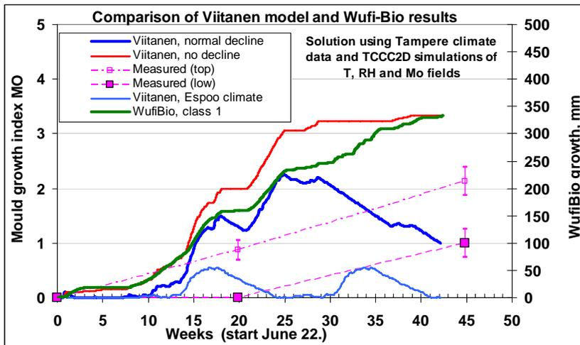
Figure 7. Comparison of VTT Model and WufiBio – and measured mould index – on pine sap wood. Results with VTT Model has been calculated under several assumptions. Viitanen, no decline is assumed to most comparable with the biogrothermal model behind WufiBio.
