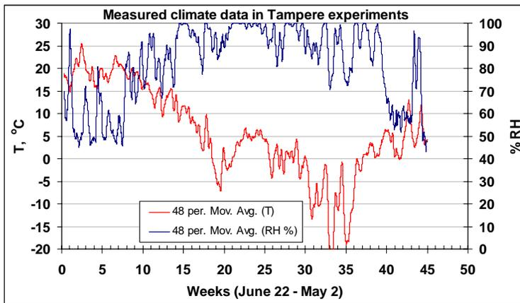
Figure 6. Measured climate data presented using 48 hour moving average values. The simulations use the original hourly measured data.
