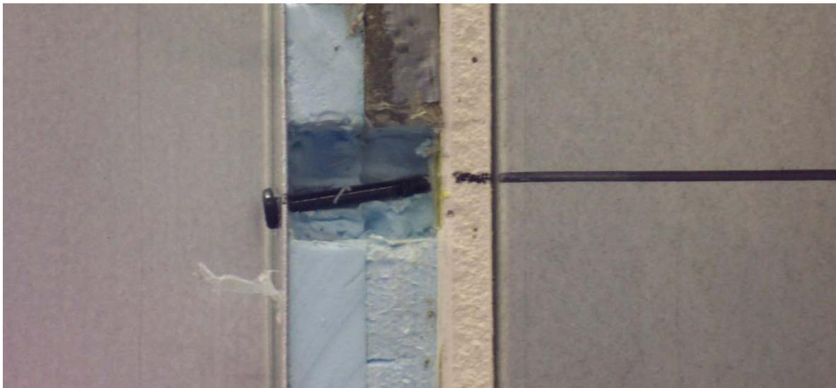
SCREW TILTING AT 50LB VERTICAL LOAD FASTENED TO 16GA STUD THROUGH 1-1/2" XPS AND GYPSUM. NOTE VERY LITTLE BENDING IN SCREW, BUT NEARLY 1/2" DEFLECTION NOTE FOAM REMOVED FOR PHOTO AFTER LOADING
