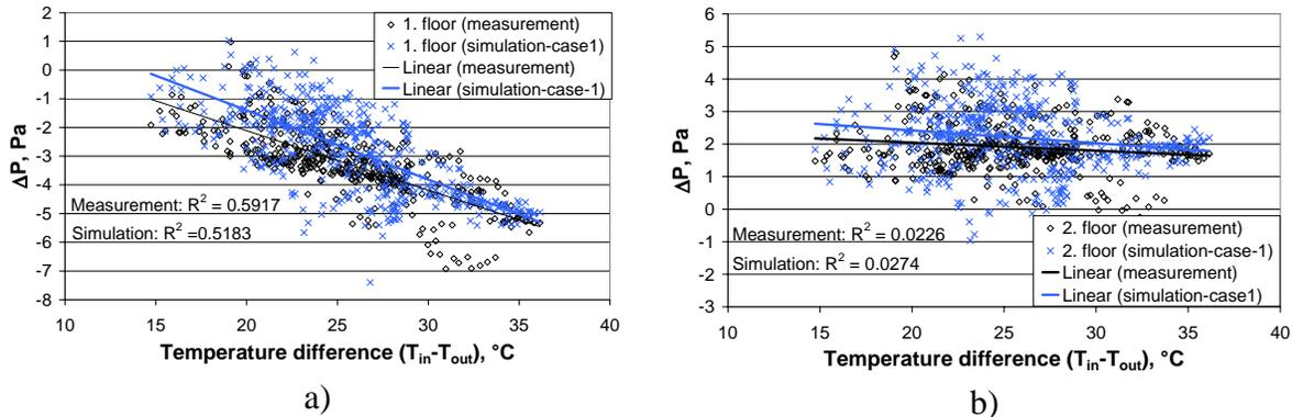
Figure 1. Measured and simulated pressure conditions of the detached house on the base (a) and top (b) floors during the test period. The pressure differences are shown as a function of the temperature difference between indoors and outdoors.
