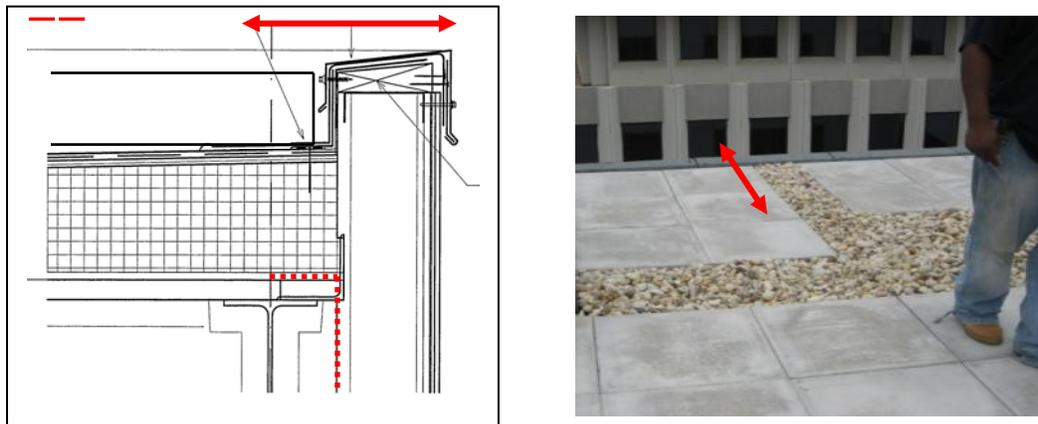
Figure 3: The Type B Zero height roof edge affords little protection with respect to wind forces. Air and thermal barrier continuity must be maintained. Rooftop users are placed at maximum personal risk along the roof edge.
