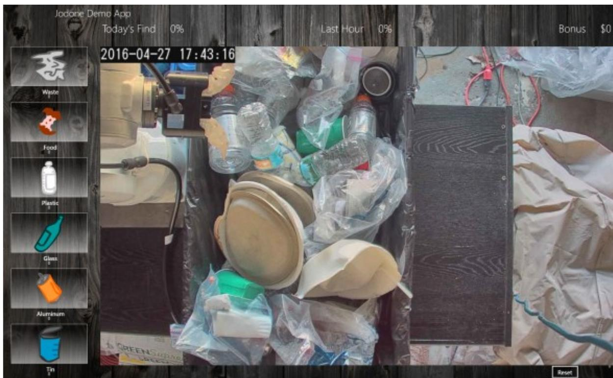
A software interface allows humans to swipe with a finger on one hand to identify trash and classify it with the other hand.
