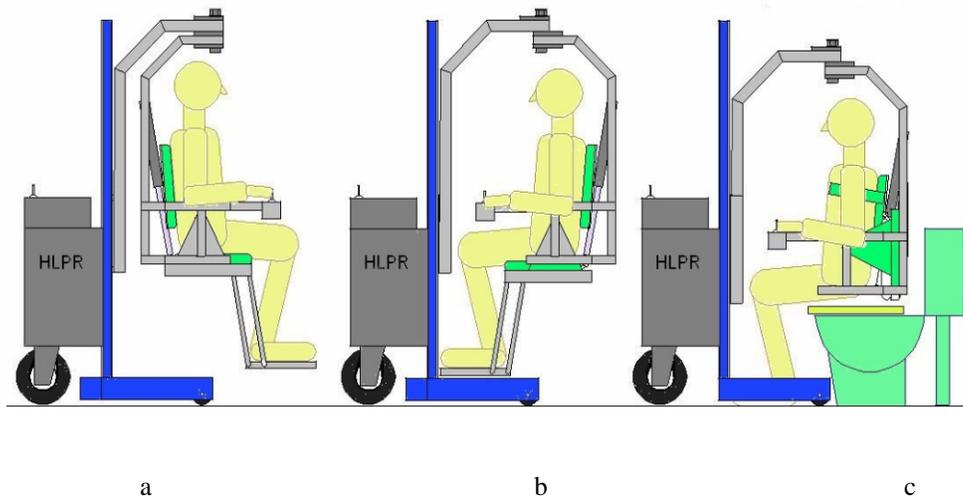
Figure 2 – HLPR Chair transferring a patient to a toilet: a) footrest has been retracted beneath the seat and the patient is approaching the toilet, b) seat frame with patient have been rotated and the seat is retracting, and c) HLPR approaches and the patient is lowering to the toilet seat.
