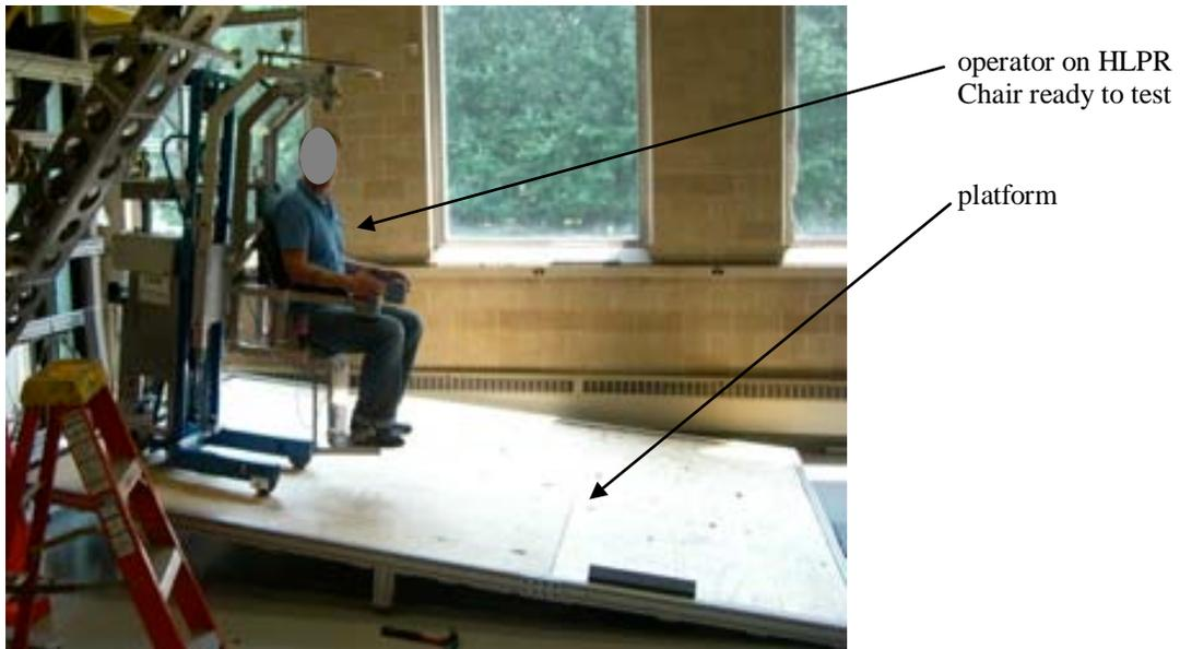
Figure 5 - HLPR chair dynamic stability test setup.
