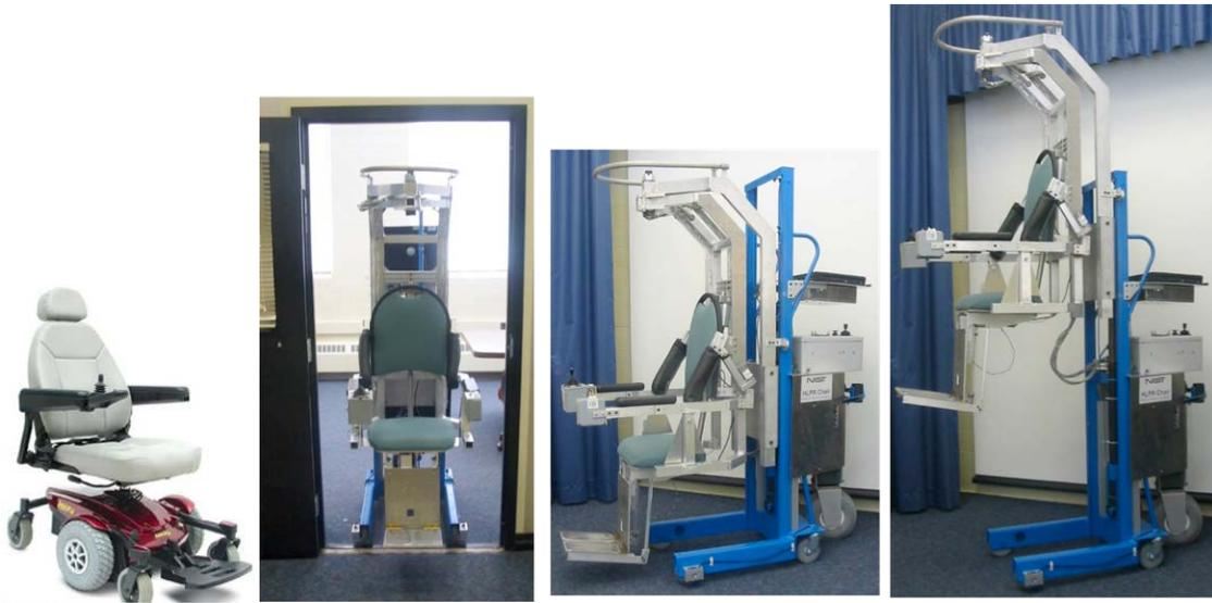
Figure 3: Typical powered chair (left) [courtesy Jazzy<sup>1</sup>] and the HLPR Chair 1 prototype (right three photos). HLPR Chair is shown in the mobility (center photos) and the lift (right-most) configurations. Note the unique shape of HLPR Chair as compared to typical powered chairs.
