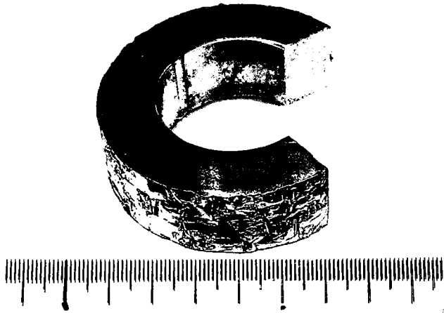
Figure 2 - Titanium deposit produced by the small scale reactor
