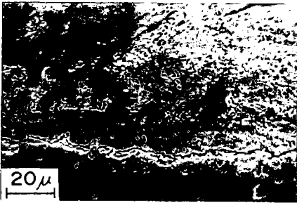
Fig.9 Ti-6Al-4V after fretting showing peripheral crack. F=500 N, P=7500 N, 1000 cycles.
