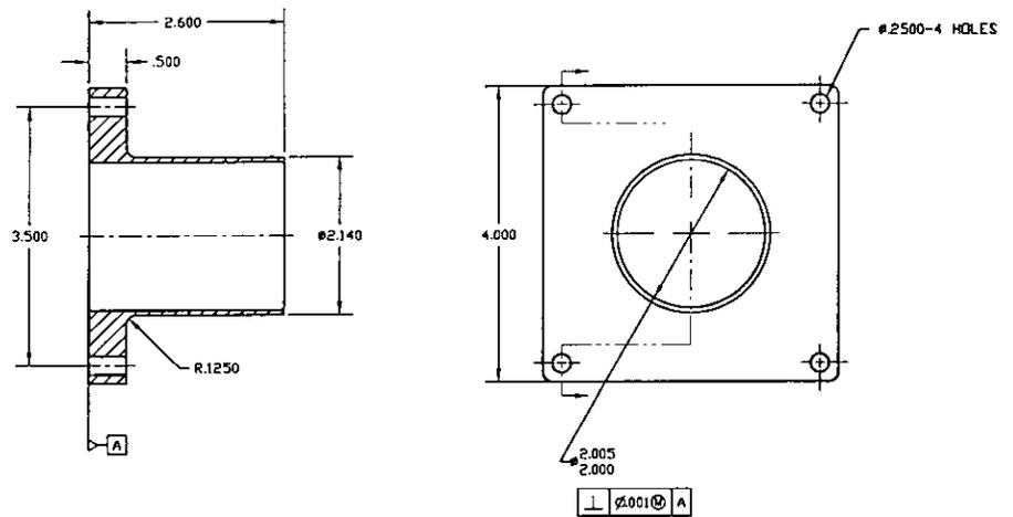
Figure 5. Perpendicularity Control.
