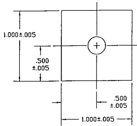
Figure 1. Conventional Tolerancing
