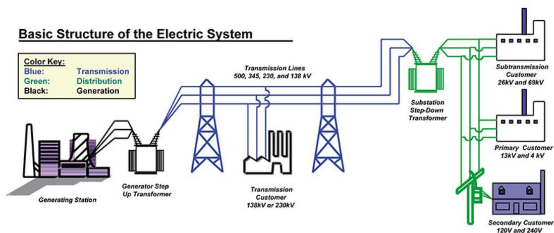
**Figure 3.** The electric grid consists of an intricate network of generation, transmission, and distribution. Customers' supply and demand for power must match exactly since energy storage is not currently widely available.
