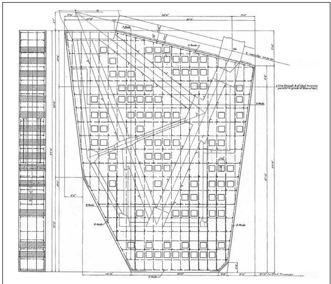
Fig. 4: Revised counterweight design for the shortened bridge, 1930
