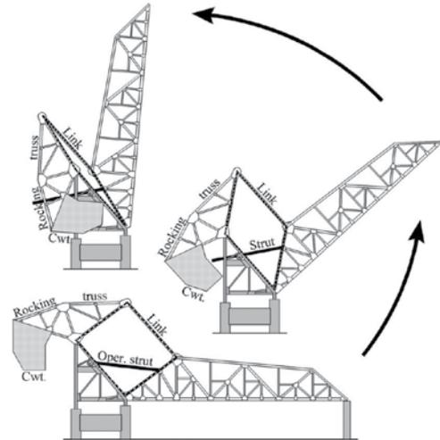
Fig. 2: Operation of the Strauss Heel trunnion bascule bridge
