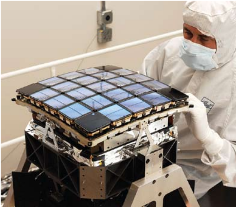
The "retina" of the Kepler photometer: a 42 CCD array with 95 million pixels. Images courtesy Ball Aerospace & Technologies Corp.
