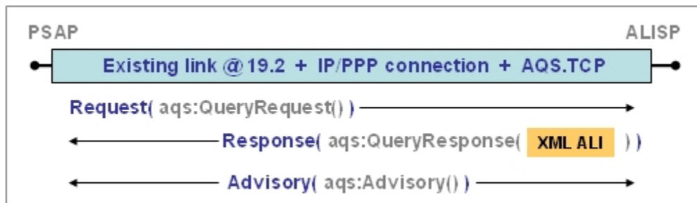
Figure 16 - Managed AQS binding (TCP version) illustration
