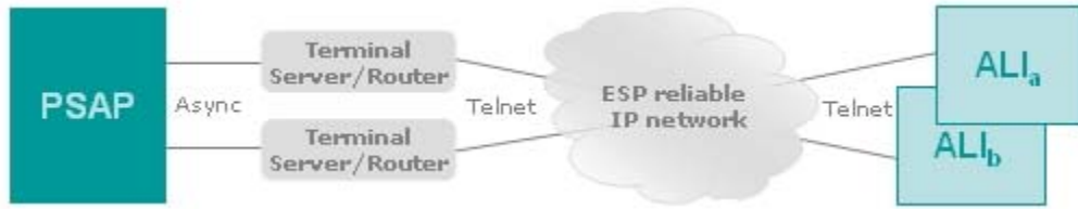
Figure 12 - IP backhaul network configuration
