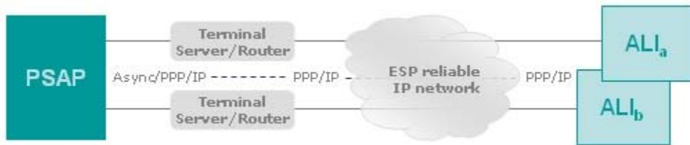
Figure 13 - PPP/IP network configuration
