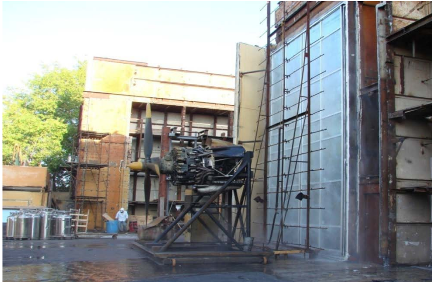
Figure 7. Dynamic water testing of a curtain wall in a laboratory. Only 5% of walls generally pass their first test.
