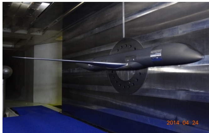
Figure 1 Half model testing in wind tunnel [3]
