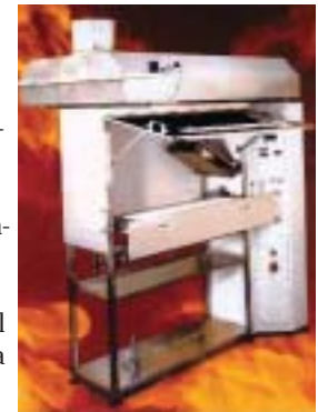
Figure 3: Flooring Radiant Panel Test Apparatus (ASTM E 648)
