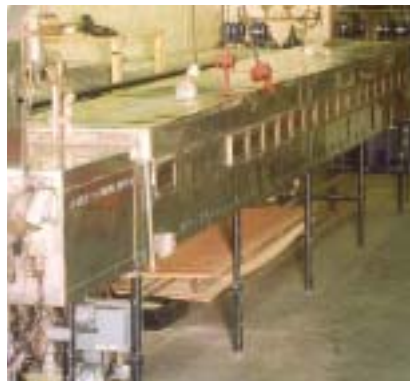
Figure 1. Photograph of Steiner Tunnel
