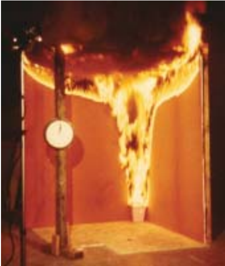
Figure 1. Open-corner test of a foam plastic insulation product with a reported flame-spread classification of 25.
